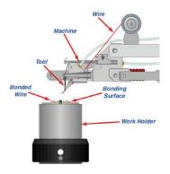
A key to wire bonding success is the original manufacturer, age, and condition of a wire-bonding tool. There are many features available with the latest semiautomatic and automatic wire-bonding machines that can dramatically increase yields, speed, and accuracy. For instance, only a few of the best wire-bonding machines enable ultra-precise dialing of the ultrasonic force, which is critical in ensuring a high-quality rapid bond.
