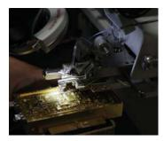
Part of the challenge for small MESA chip wire bonding, is that every MESA chip may have significantly different requirements for the optimum wire bond. Balancing cost, performance, time, yield, and process development is becoming overwhelming for many manufacturers. To deliver the best quality bonds that meet stringent application-specific evaluation parameters and standards, the customization of wire-bond tools is often necessary.
