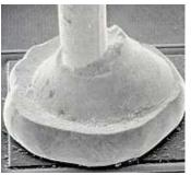
Due to the high pressures and heat involved with thermocompression, which also impacts thermosonic wire bonding to some degree, cratering and peeling of the wire bond pad is possible. This failure mode may lead to increased resistance from the die to the package, and lead to heat stress and performance issues with high-speed signals. Cratering and wire-bond peeling can also result in complete disconnection over time and stress.
